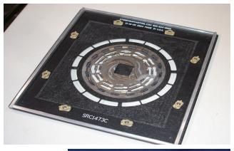
Titanium inserts are used when only partial areas of a PCB have spacing too close for a composite only pallet base. Inserts can range in size and can be basic or complex depending on the PCB layout and process needs.
