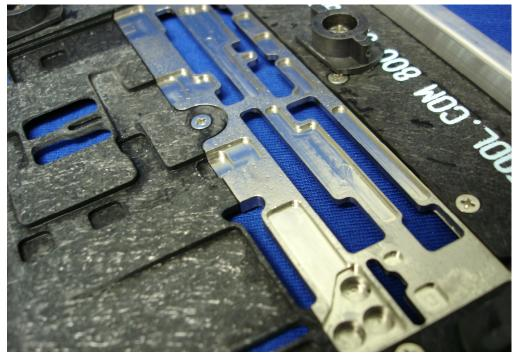
Titanium fixtures are used during a selective solder process when the through hole lead is too close to a bottom side SMD to use a standard composite sealing wall. While the titanium allows several superior qualities such as rigidity, intricate thin wall machining
