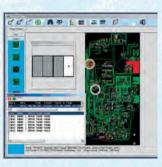
The VIVA software includes a graphical repair environment, which enables the user to locate and view the parts of the PCB which have failed during the test, facilitating repair operations.
