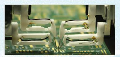
Component Test: The **RAPID NEXT**>**SERIES** systems can generate and perform all of the parametrical and functional tests of passive and active embedded components, thanks to Seica's decades of experience and technology developed for full, loaded board tests.
